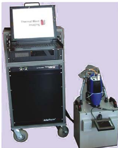
Fig.2. Photograph of pulsed thermography system
