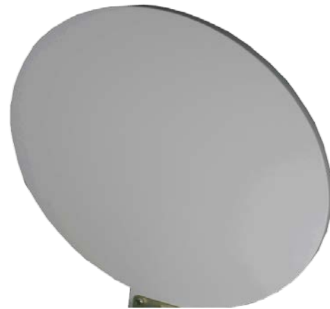
Fig.10. Circular parabolic honeycomb structure
